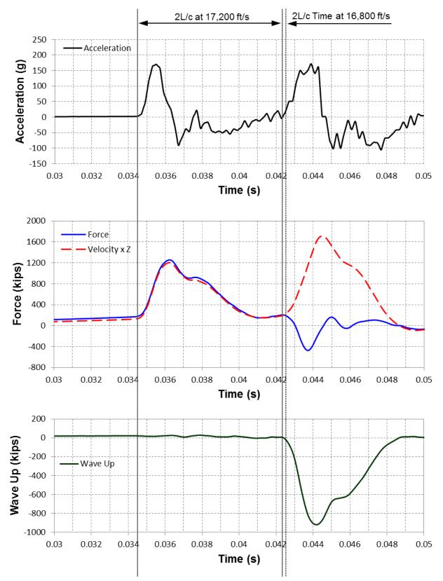
Figure 4. Case 2 – Acceleration (top), Force and Velocity Records (middle) and Wave Up (bottom) for Blow 6 in Early Easy Driving Conditions. Wave Speed of 17,200 ft/s (5,243 m/s).
