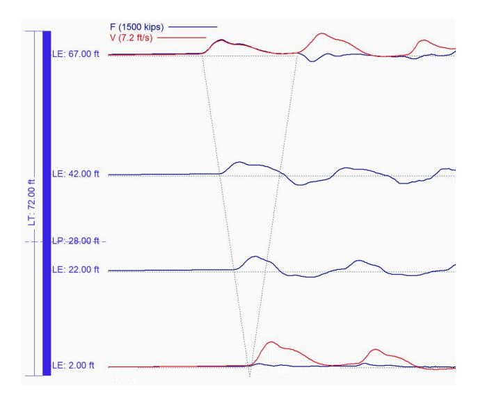
Figure 3. Case 2 - Wave Travel Past Multiple Gage Locations at Wave Speed of 17,200 ft/s (5,243 m/s).
