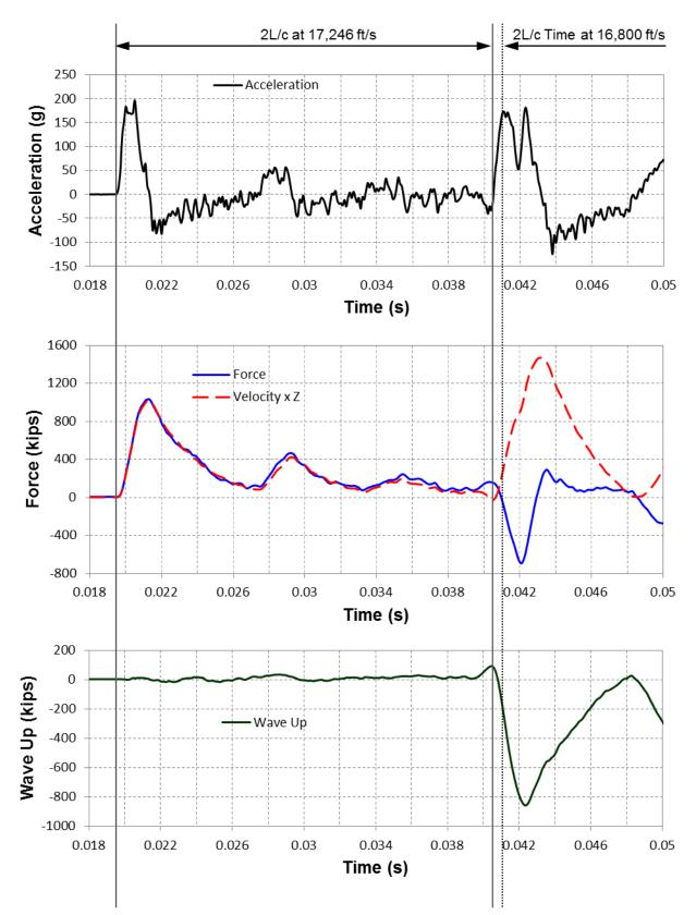
Figure 5. Case 3 – Acceleration (top), Force and Velocity Records (middle) and Wave Up (bottom) for Blow 2 in Early Easy Driving Conditions. Wave Speed of 17,246 ft/s (5,257 m/s).
