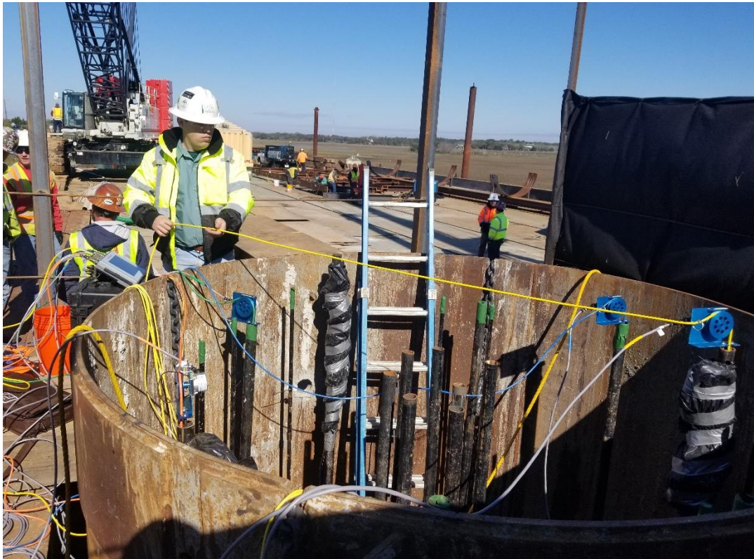
Figure 5. Cross-hole Sonic Logging Test Using Multiple Transceivers.
