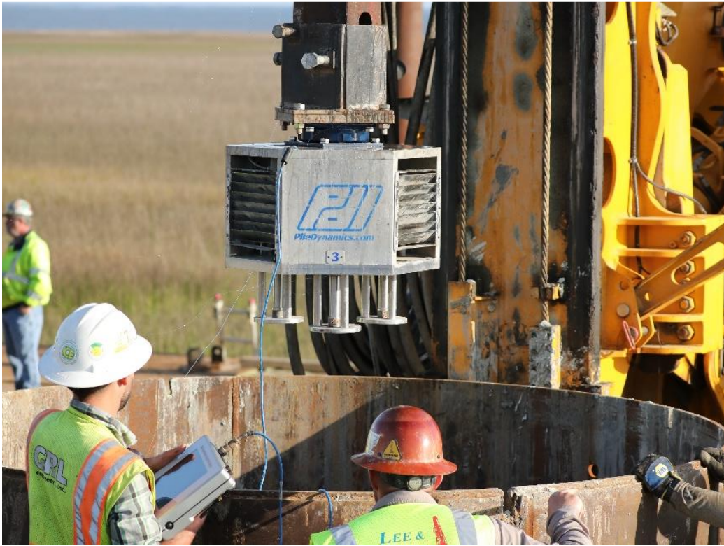
Figure 3. Shaft Quantitative Inspection Device.
