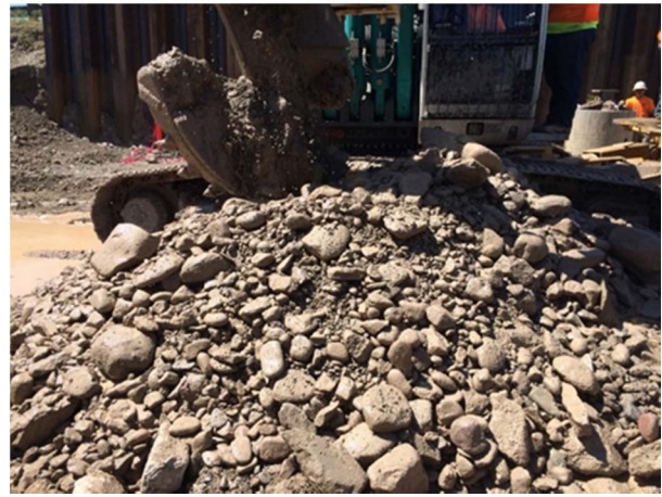
Fig. 3. Typical subrounded to subangular poorly graded gravel, with sand, cobbles, and boulders (from 40 feet)
