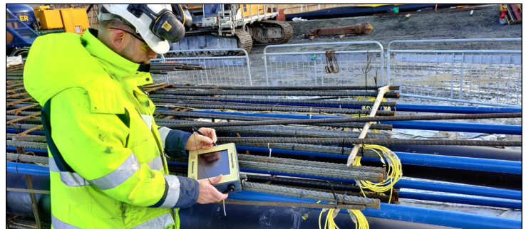
Image 3. Thermal Integrity Profiling for Mass Concrete
