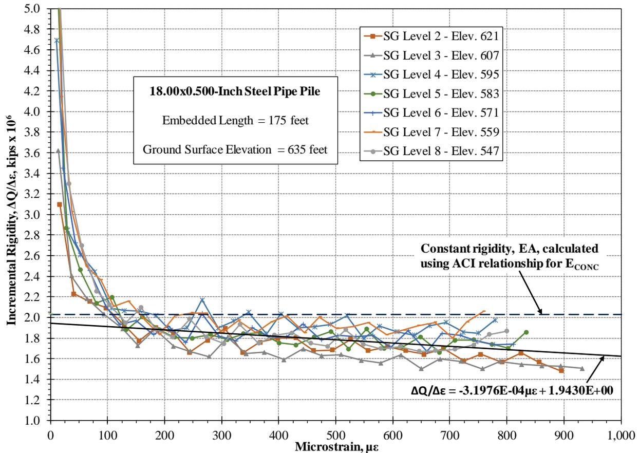
Fig. 7. Incremental rigidity diagram for those strain gage levels that showed similar IR relationships, illustrating selection of a single best-fit trend line.
