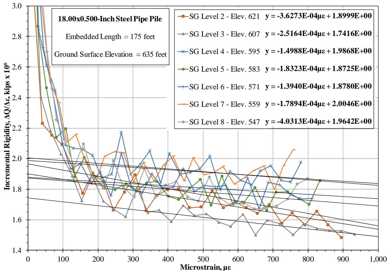
Fig. 10. IR diagram illustrating individual relationships for SG Levels 2 through 8.
