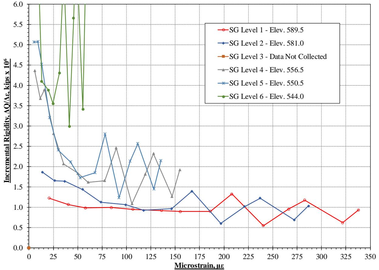
Fig. 5. Illustration of the effect of using single test load and strain values.
