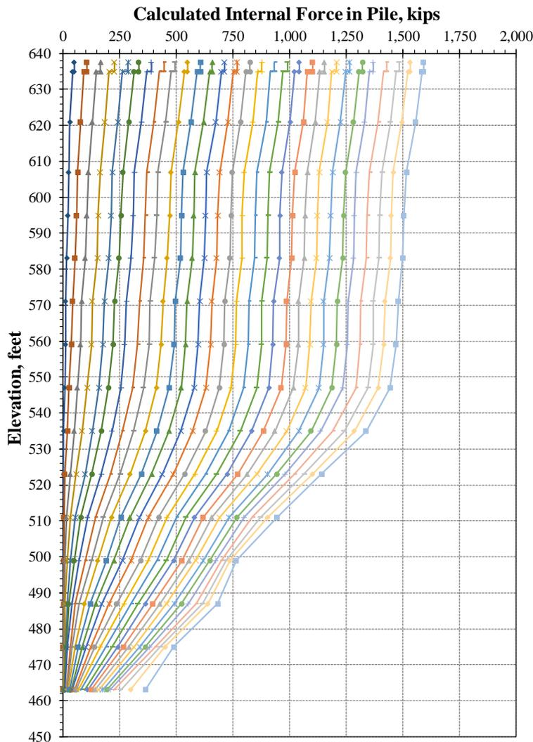
Fig. 11. Internal force profiles determined using individual incremental rigidity relationships for each strain gage level.
