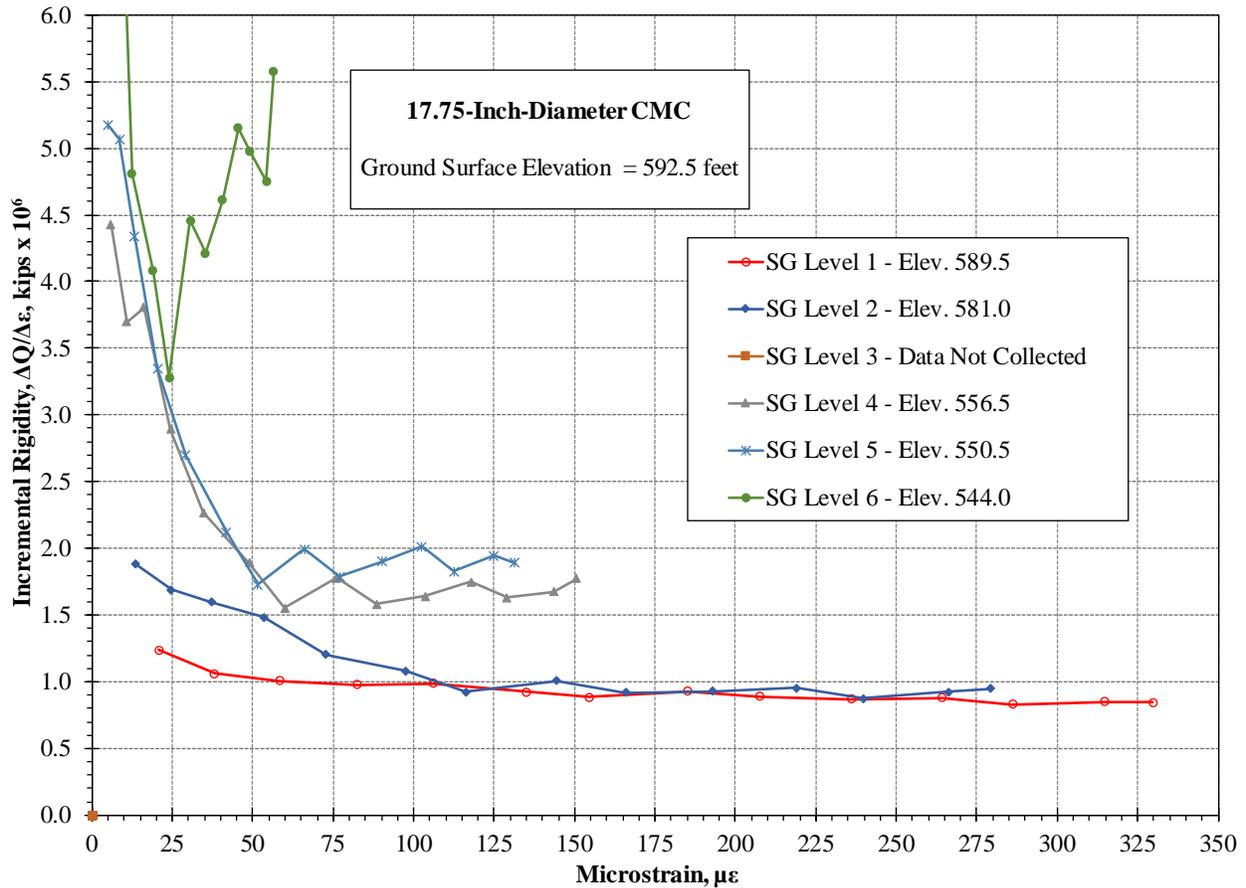
Fig. 4. Illustration of non-interpretable strain gage levels as a result of pile-end displacement, and the effect of using average test load and strain values.
