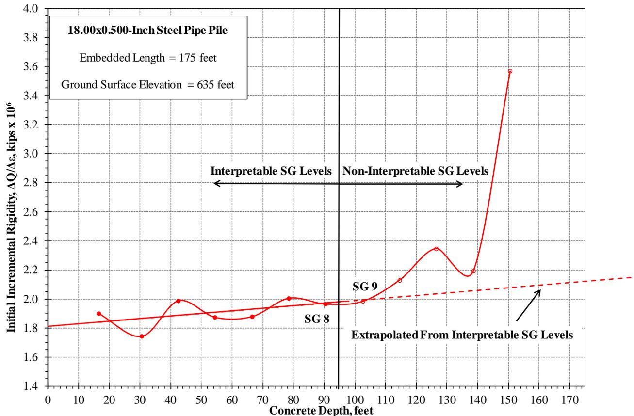
Fig. 12. Initial incremental rigidity values versus concrete depth.
