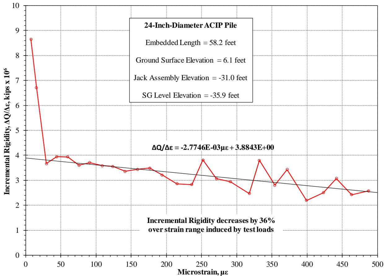
Fig. 1. Incremental rigidity plot for one strain gage level depicting significant decrease over strain range induced during static loading test.
