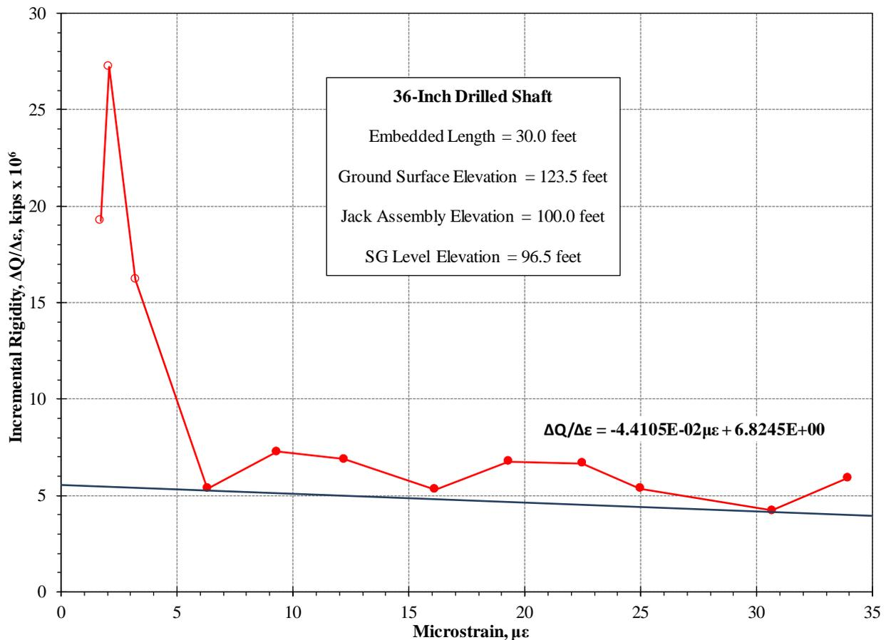
Fig. 2. Incremental rigidity plot for one strain gage level exhibiting linear response at relatively low strain magnitudes.
