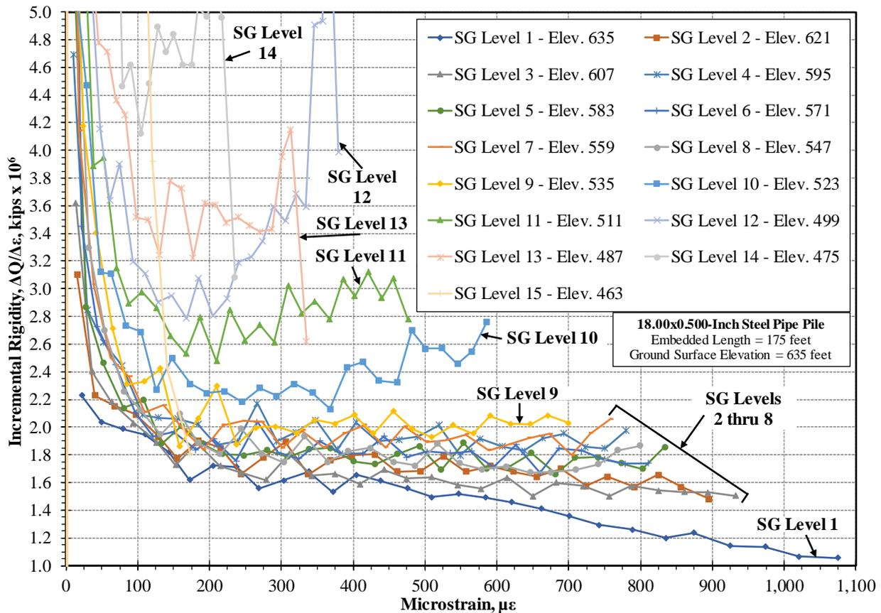
Fig. 6. Incremental rigidity relationships for all strain gage levels in a 175-foot-long concreted-in-place pipe pile.
