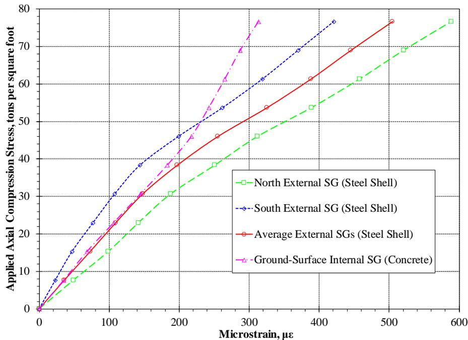
Fig. 3. Illustration of concrete fill and steel shell de-bonding during a head-down static loading test in a concreted-in-place pipe pile.
