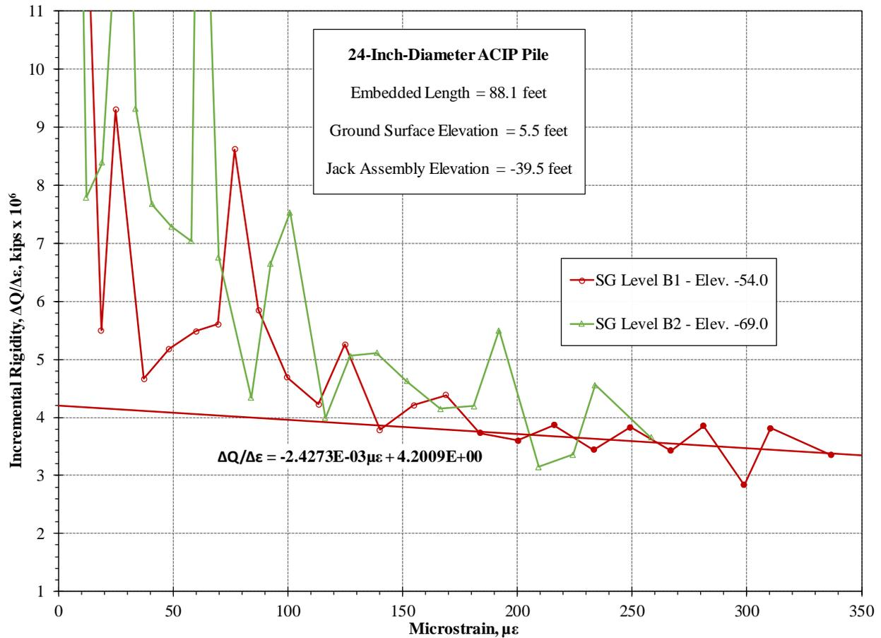
Fig. 13. Similar incremental rigidity relationships exhibited by strain gage levels with apparently different cross-sectional areas.
