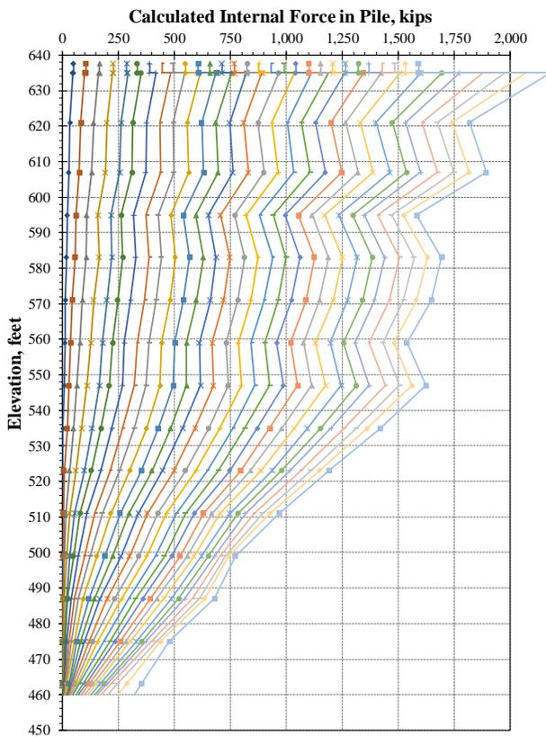
Fig. 8. Internal force profiles determined using a constant rigidity,  $EA$ , calculated using ACI relationship for  $E_{CONC}$ .
