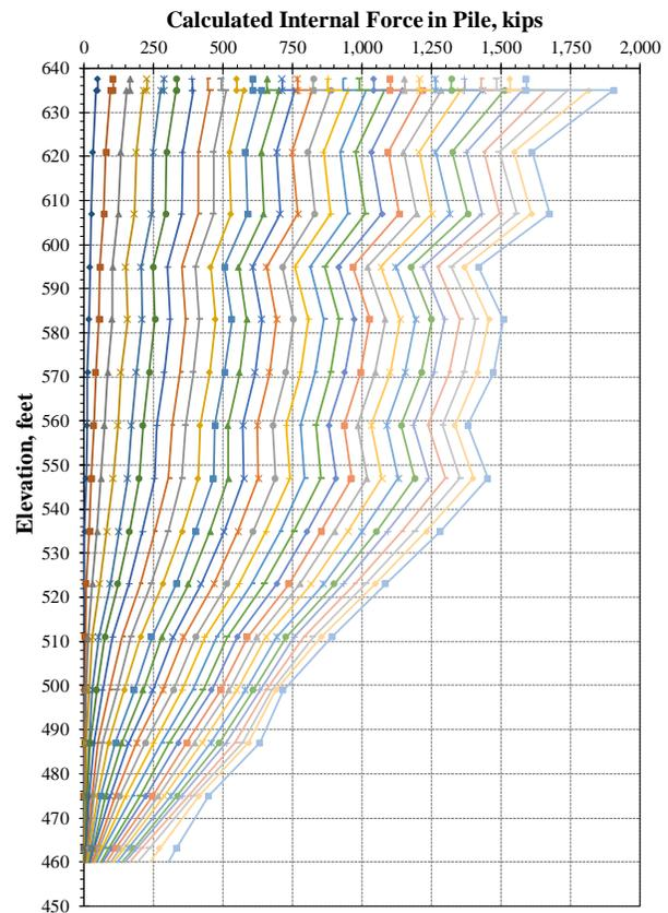
Fig. 9. Internal force profiles determined using a single best-fit strain-dependent incremental rigidity relationship.
