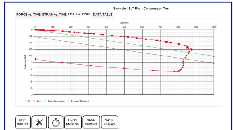
Load vs Displacement report on a recent Static Load Test
