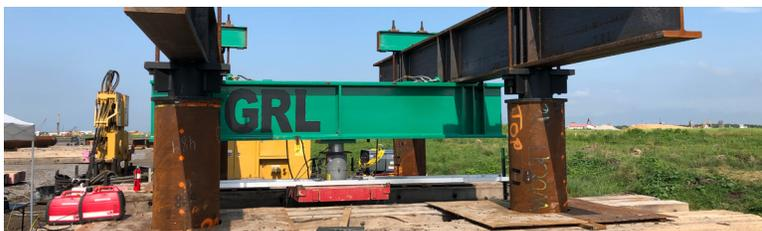
GRL performed a SLT with GRL's 500 ton frame on a 30-inch (76.2cm) open-ended pipe pile for the Calcasieu Pass Liquefied Natural Gas (CPLNG) project.
