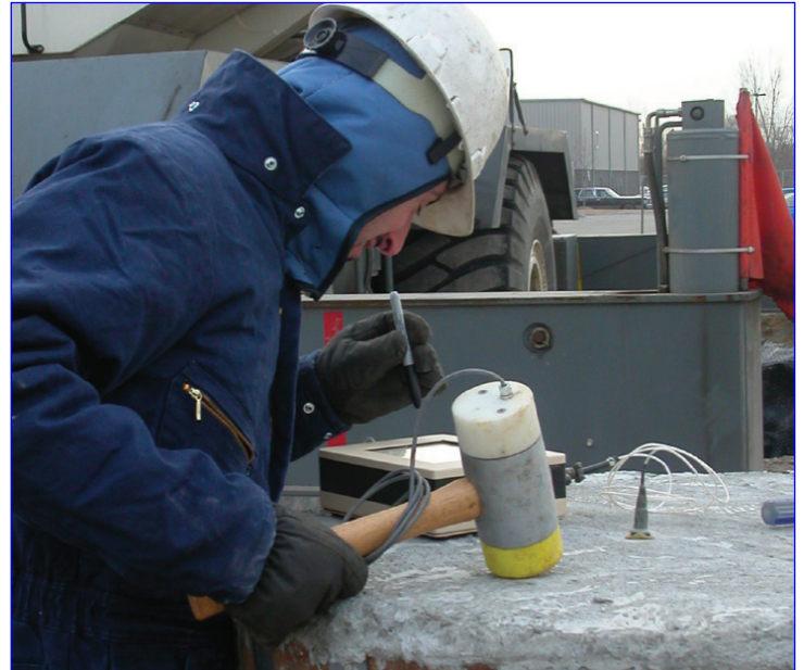
GRL Cleveland office manager C. Michael Morgano applies PIT to a 4ft diameter drilled shaft
