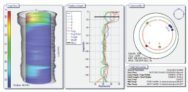
Figure 1: TIP Reporter screen shot. On the left is a 3D image of the effective shape of the shaft that can be rotated to any orientation. The center image plots effective radius versus depth. On the right, a "horizontal slice" shows the inner cage radius (inner circle), the nominal shaft diameter (middle circle), and outer shaft profile (outer circle). The slice is from the upper, temporary cased portion of the shaft; its location is indicated in the center image by a horizontal line.
