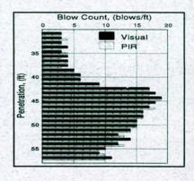
The *Driven PIR* (for impact driven piles) has already been tested on several sites. (See chart for a comparison of visually and PIR-automatically measured-blow counts.) The PIR is capable of accepting additional channels of information such as pile inclination, pile rebound, *etc.*, thereby providing for a complete pile installation record.
