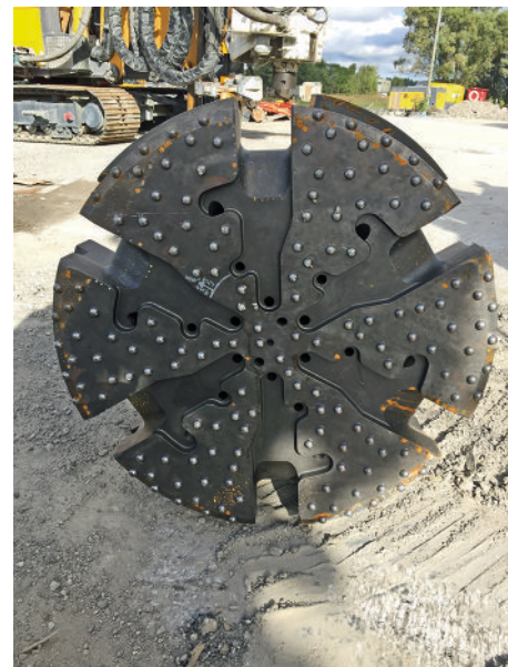
(L) Button driving ring at tip of pipe pile and (R) bottom of a DTH to fit inside pipe pile
