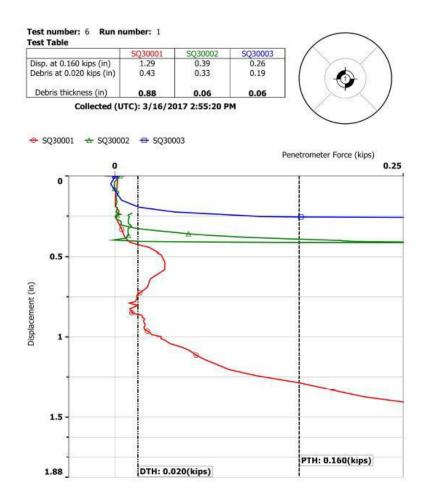
Figure 4. Force vs. displacement plot with debris thickness determination from SQUID test
