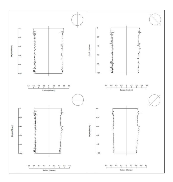
Figure 5. Ultra-sonic profiling output from SHAPE device
