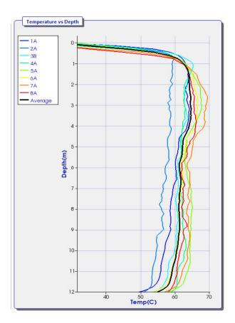
Figure 3. Thermal results showing cage eccentricity
