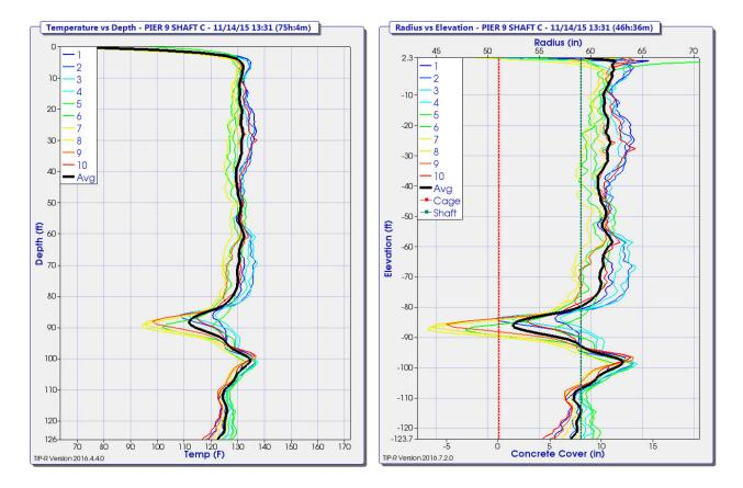
Figure 2. Thermal results of temperature vs depth (left) and radius vs elevation (right) for the same drilled shaft with a defect at 27.4 m (90 ft.)
