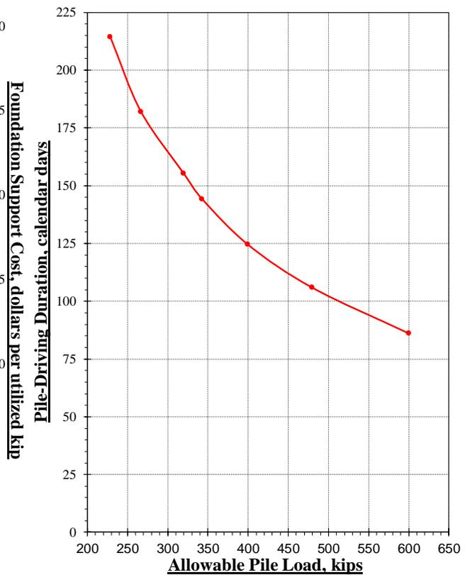
**Figure 3. Driving Duration vs. Allowable Pile Load.**
