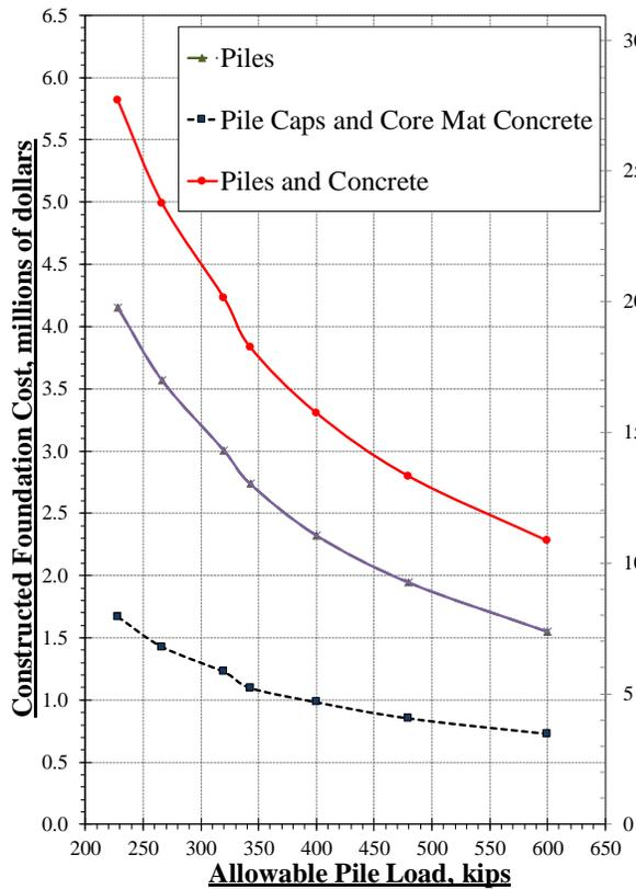
**Figure 2. Constructed Foundation Cost, and Foundation Support Cost, vs. Allowable Pile Load.**
