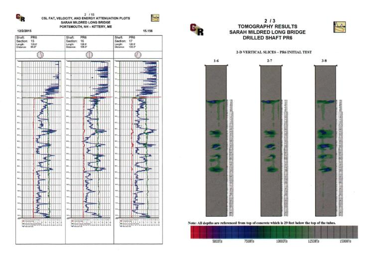
Figure 12: CSL Test Results and Tomography Results (Geosciences Testing and Research, Inc.).
