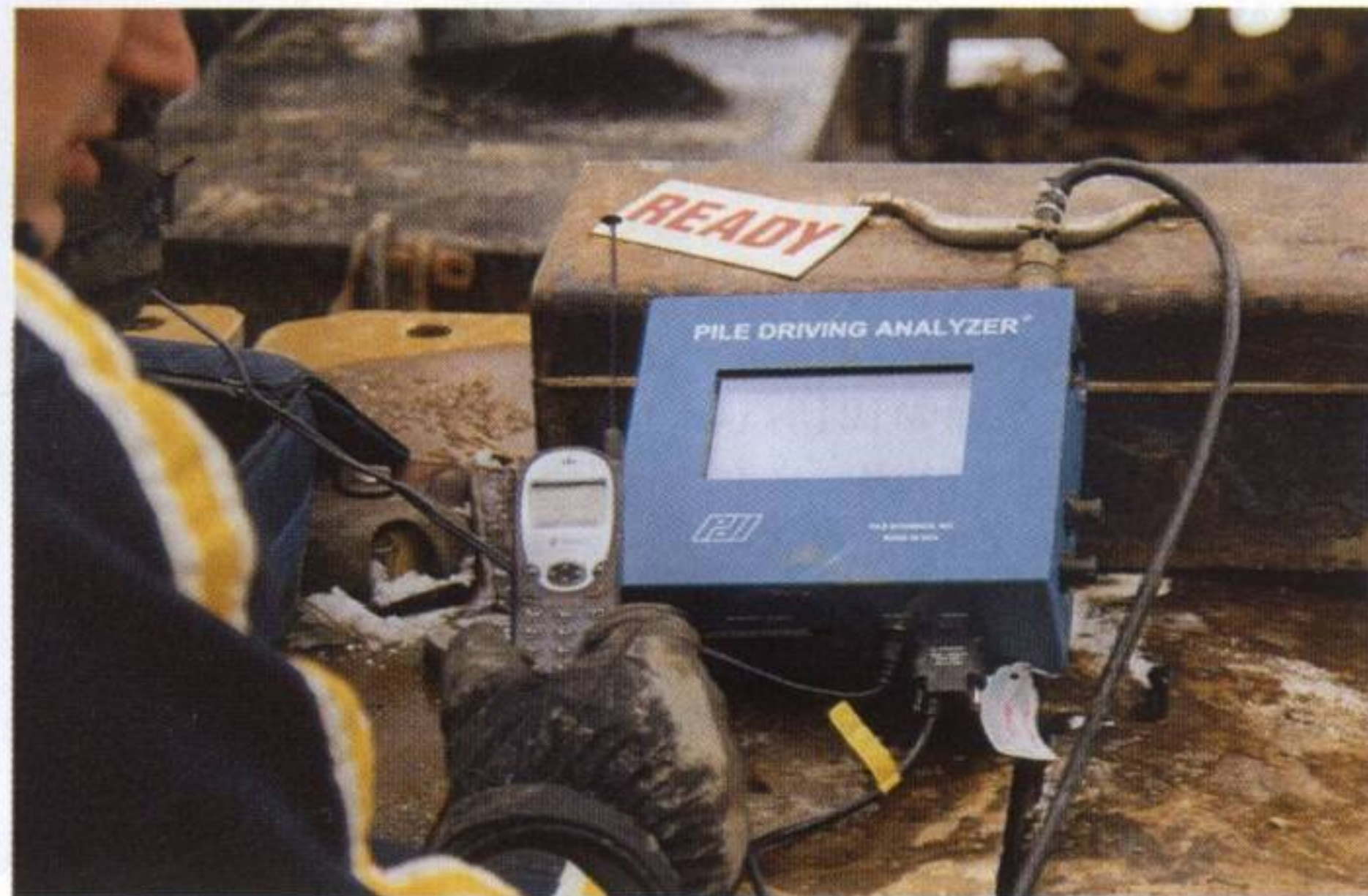
The PAL-R from GRL Engineers Inc. is a Pile Driving Analyser (PDA).
