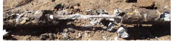
Figure 6: 100% Loss in Section Coverage
