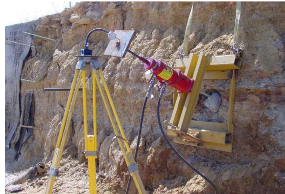
Figure 3: Jack and Reaction Frame
