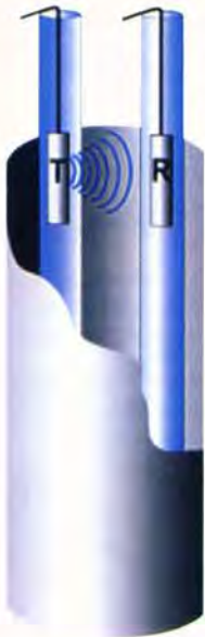
Figure 7: A schematic drawing of cross-hole sonic analysis.
