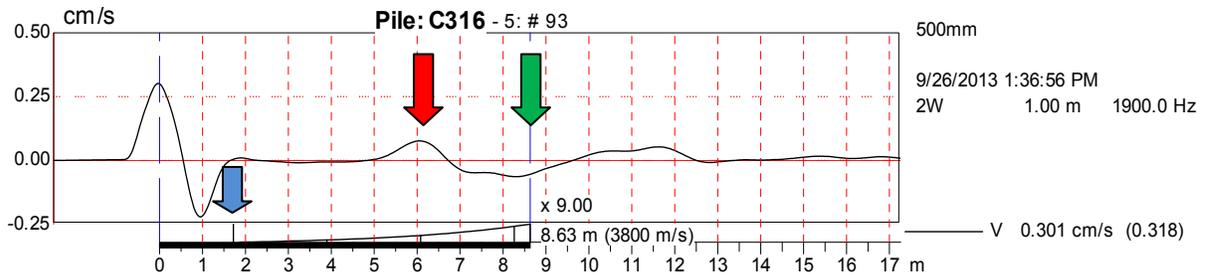
Figure 7 Appropriate MD – Defective Pile
