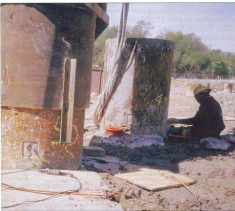
PDA instrumentation on a 1,200mm diameter drilled shaft in preparation for a test with a 25 tonne ram with 2,000 tonne test load.
