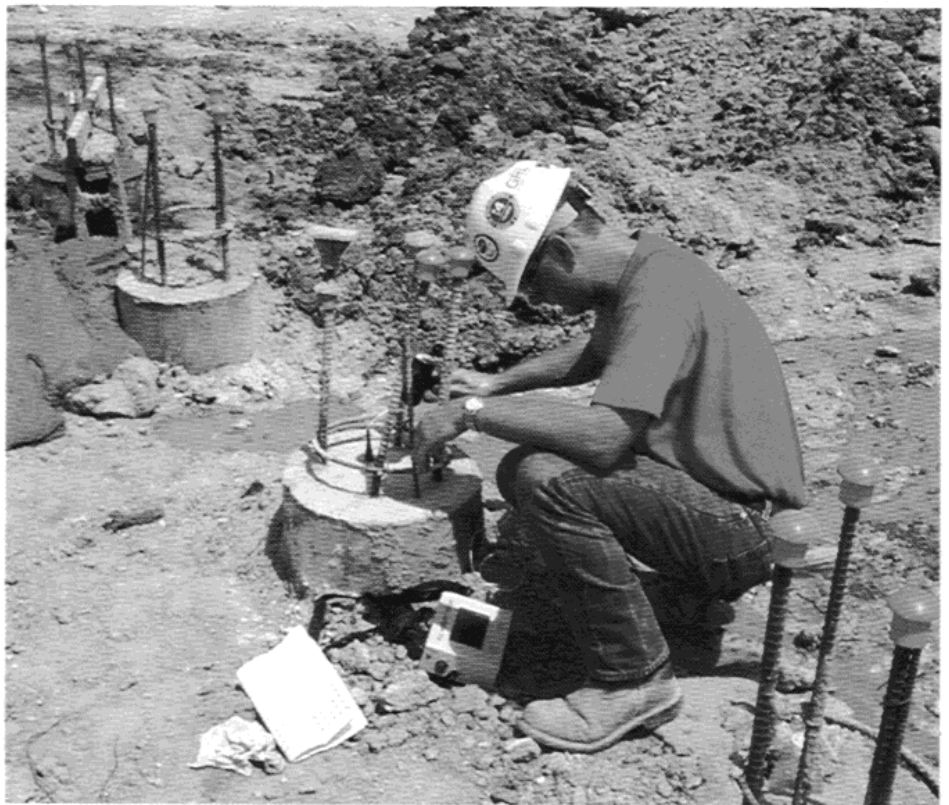
Surface Reflection Integrity Testing.
