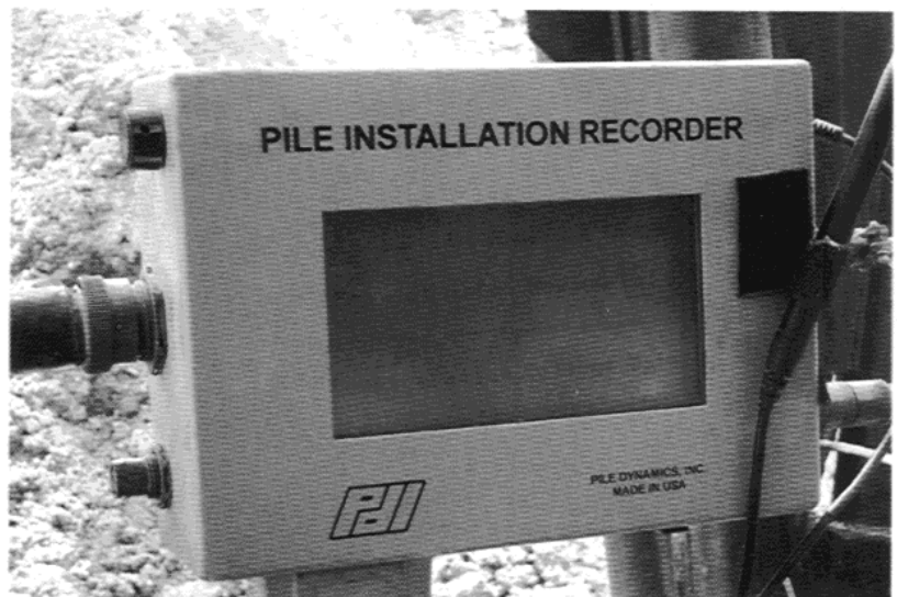
Main Control Unit for PIR-A Monitoring Equipment.
