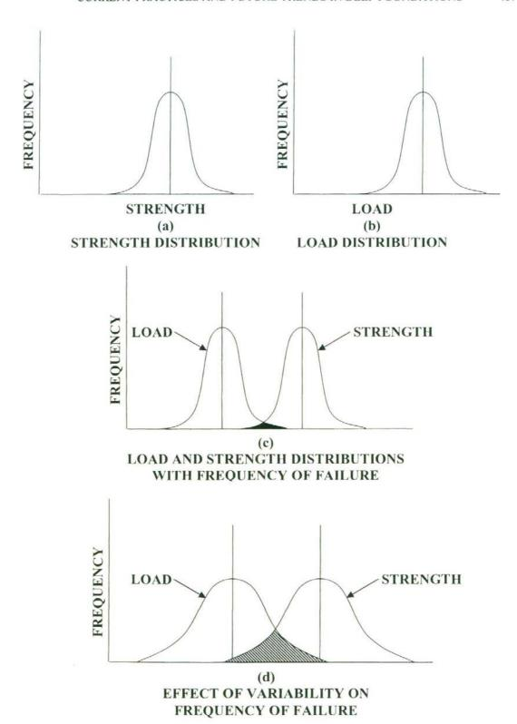
FIG. 1. Effect of variability of distribution of load and strength on frequency of failure
