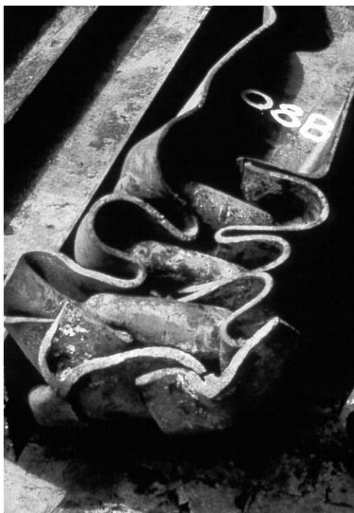
Figure 1. Damaged H pile.
