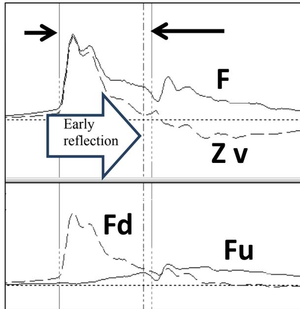
Figure 10. Pile driven to 78 ft (23.8 m) demonstrates near-toe damage.
