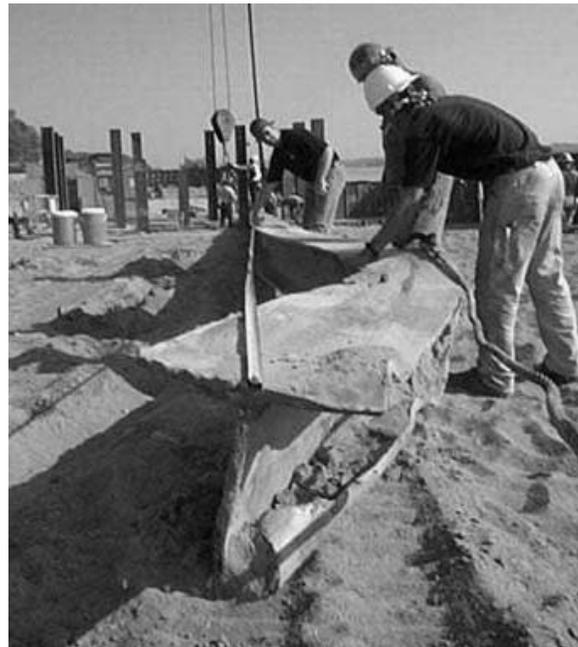
Figure 11. Extracted pile with near-toe damage.
