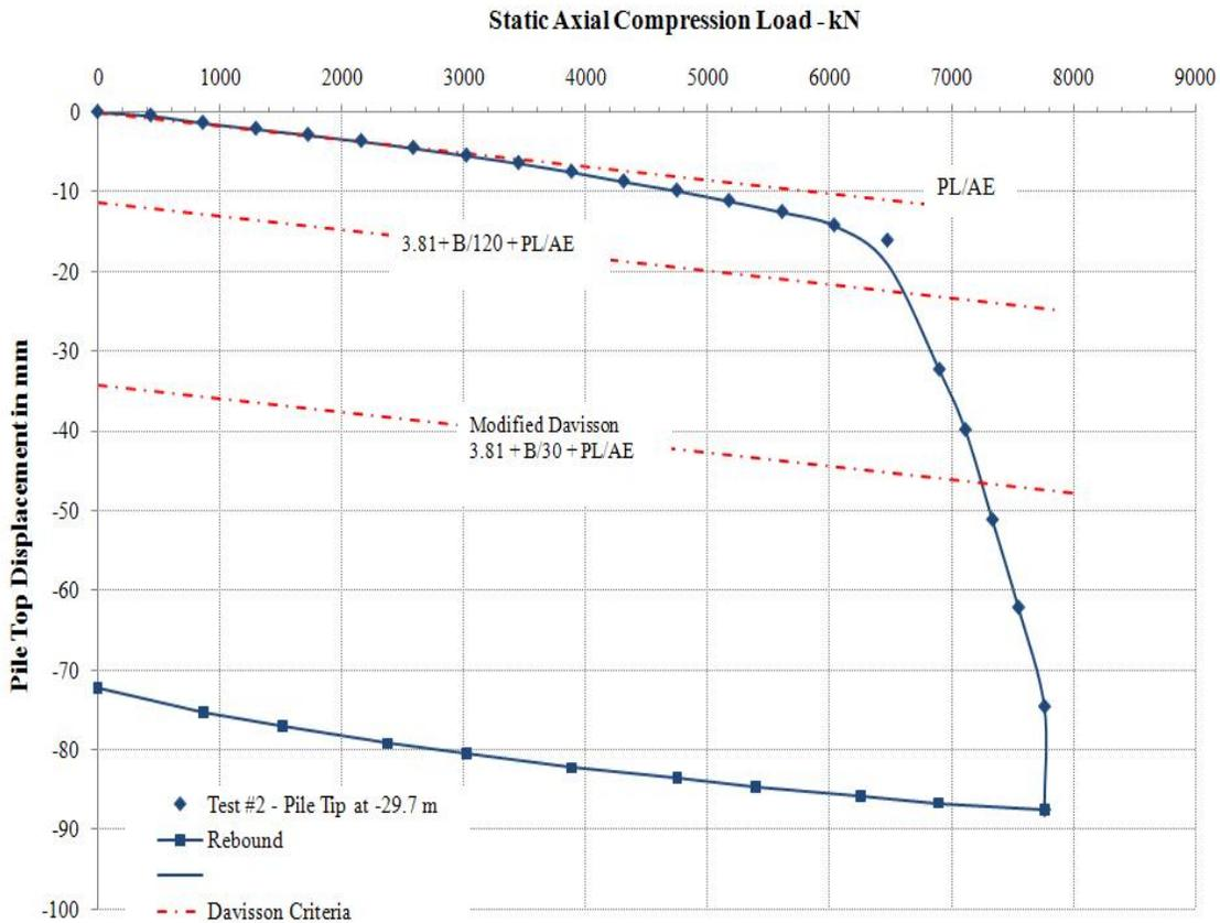
**Fig. 8 Results of the second static loading test.**
