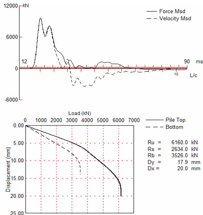
**Fig. 6 PDA and CAPWAP testing and analyses results for end of driving.**
