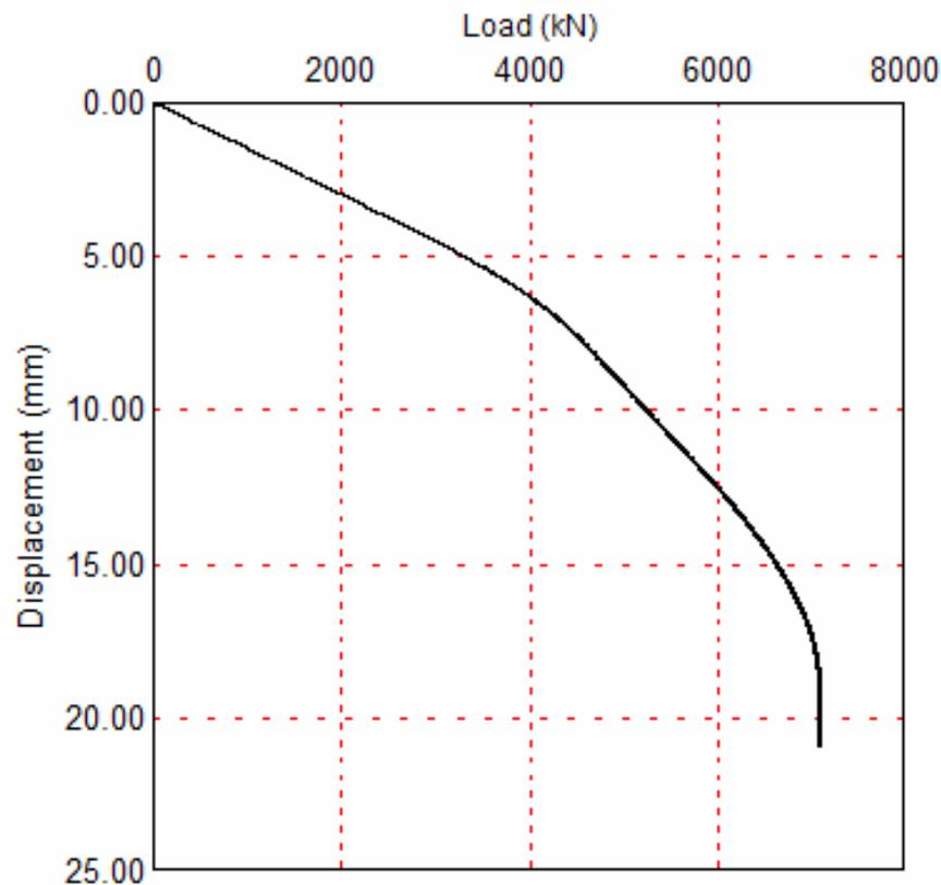
**Fig. 7 CAPWAP simulated pile top load-movement relationship incorporating end of driving results and anticipated increase in pile capacity.**
