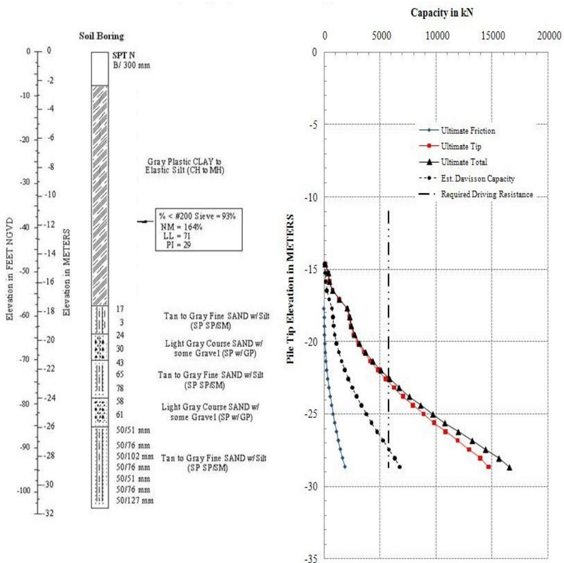
**Fig. 1 Soil boring and geotechnically calculated pile capacities.**
