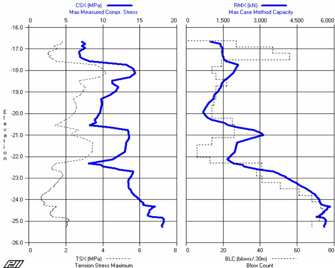
**Fig. 2** Pile initial driving dynamic testing results.
