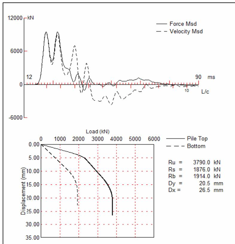
Fig. 5 Dynamic testing results of pile restrike test after static loading test.
