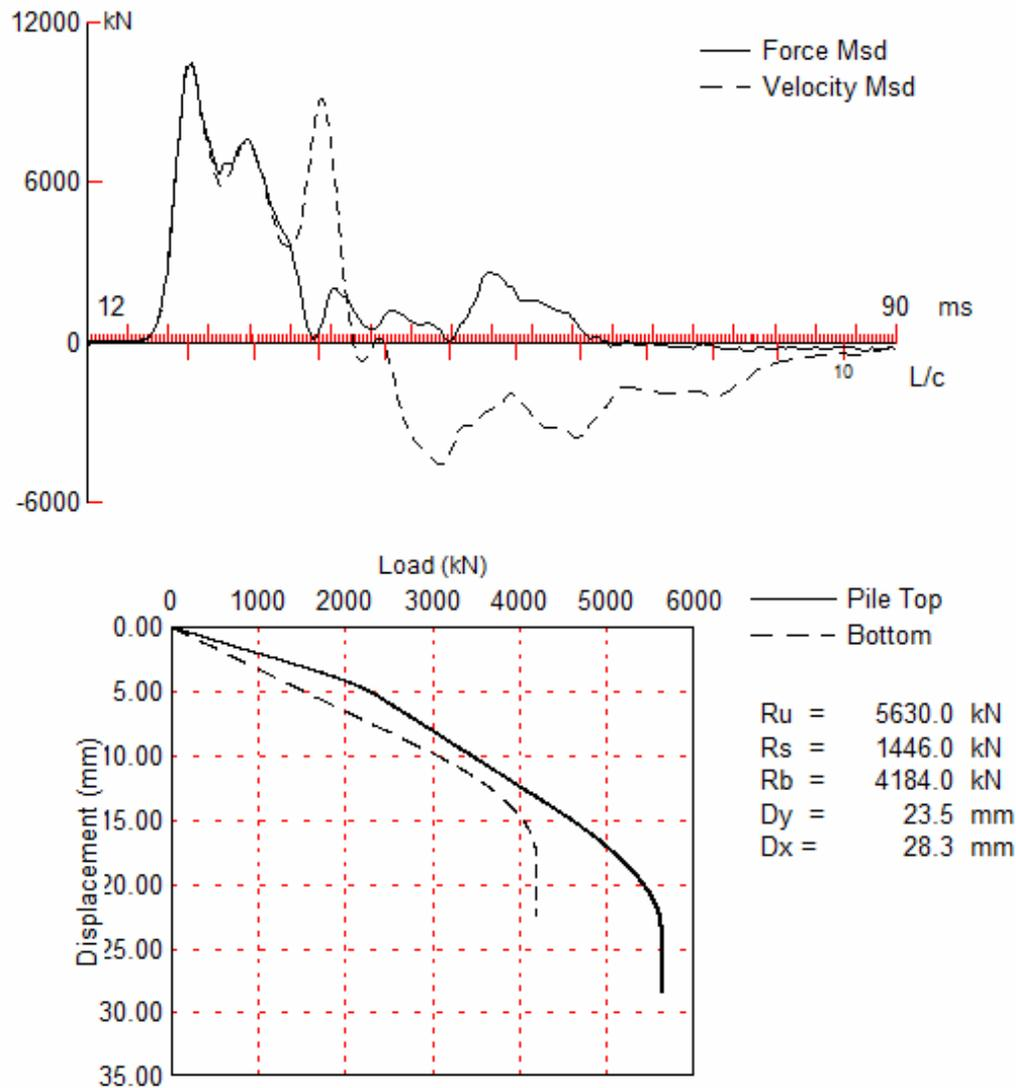
Figure 3 CAPWAP analysis results for end of initial driving.
