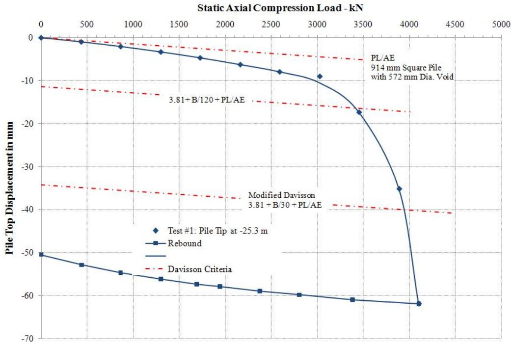
**Fig. 5** Results of static loading test.
