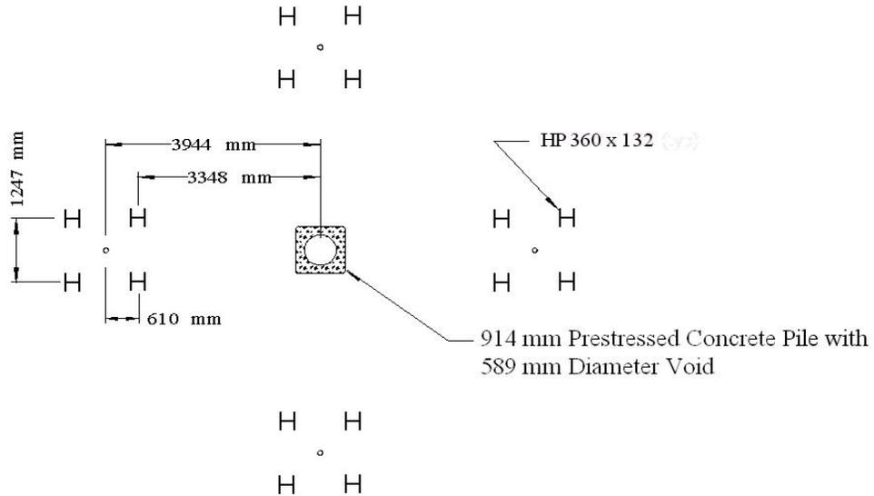
**Fig. 4** Layout of test pile and reactions piles.
