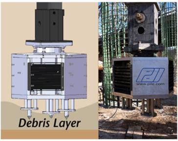
Figure 1. SQUID penetrometers penetrate the debris layer
