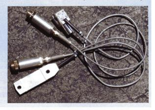
**GRL Engineers, a US-based** specialist in deep foundations testing, has equipped all its offices with Pile **Dynamics' new Pile Driving Analyser** (PDA), the PAL-R. which transmits pile testing data via a cell phone to the engineer's office where it can he monitored in real time
