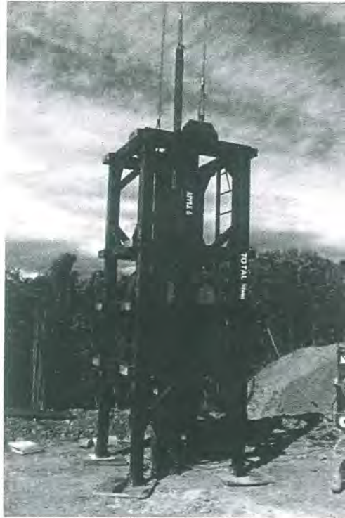
Figure 3. Stock photo of the APPLE VI Dynamic Load Testing System.
