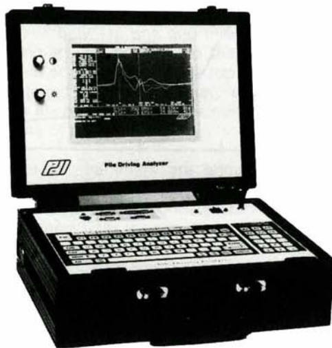
Figure 2: The Pile Driving Analyzer
