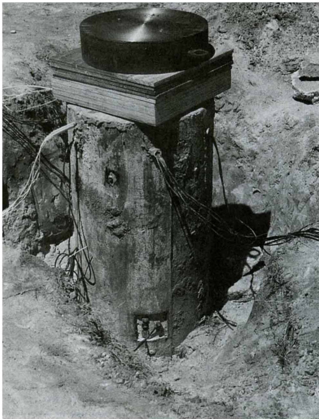
FIGURE 4 Clockwise from top left: Pileco 19.5-kip ram, GCPC Pile Driving Analyzer PIT low strain testing, instrumented pile, and cushion and striker plate.
