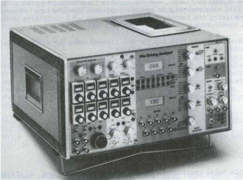
Figure 6: Pile driving analyzer .
