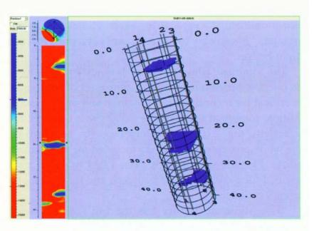
Pile Dynamics, Inc., a leading manufacturer of quality assurance equipment for the foundation industry, has developed exciting new enhancements for its Cross Hole Analyzer (CHA), a device to inspect drilled shafts and other cast in place piles for defects utilizing the cross-hole sonic logging method:
