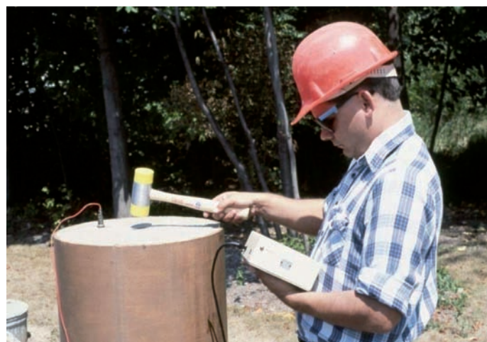
Figure 2. Low Strain Integrity Testing.
