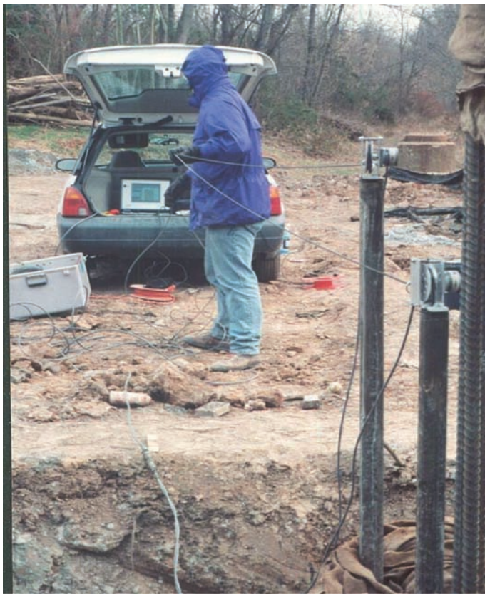
Figure 1. Cross-Hole Sonic Logging.
