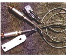
bility of human error when entering the calibration factors, according to Pile Dynamics. Just connect these new accelerometers and strain transducers to the PDA and the PDA automatically knows to which channel each Smart Gage is connected, the gage number, its calibration, and date of last calibration. The date of last calibration serves as a reminder to recalibrate the gages every two years in order to maintain data accuracy.
