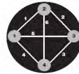
Shaft cross section with four tubes, six paths are tested.
