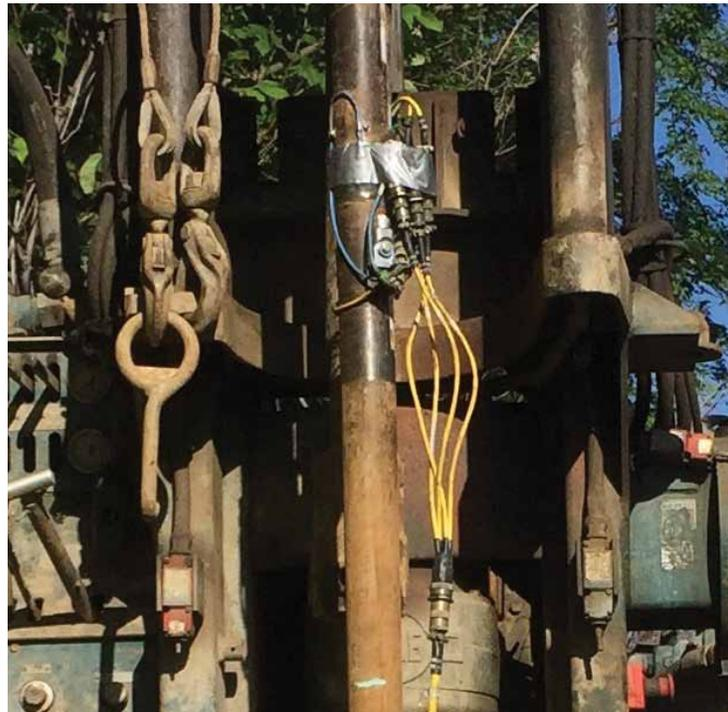
*SPT hammer in the process of being calibrated with SPT Analyzer - notice instrumentation on the drill string*
