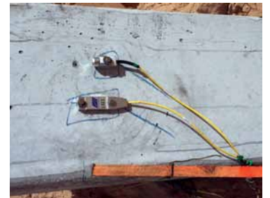
Traditional (cabled) accelerometer and strain transducer
