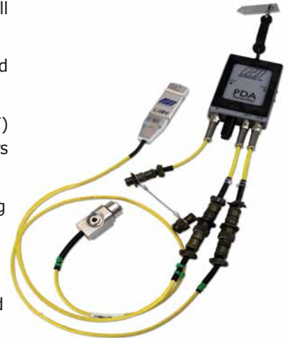
clockwise from top: wireless transmitter, accelerometer and strain transducer
