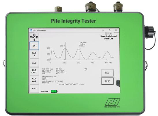
corresponds to the pile length. If a defect is present along the shaft, its size and location affect the propagation and reflection time of the wave.
