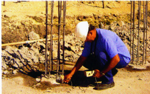
Use of Pile Dynamic's Pile Integrity Tester (PIT) at a wind farm project in Brazil is helping to speed up the checking process and allow turbine erection to progress.
