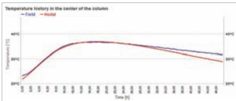
*Tempjet software output: measured temperature histories (temperature versus time) in a jet-grouted column. Each line indicates the temperature history measured by one sensor*
