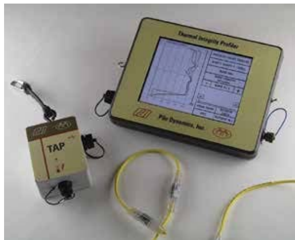
Pile Dynamics Inc.'s thermal integrity profilers track the temperature inside cement piles to ensure they were poured properly, thereby ensuring the structural integrity of the project. Data are collected for the 28-day curing period on the digital monitor, left above ground and later disconnected.
