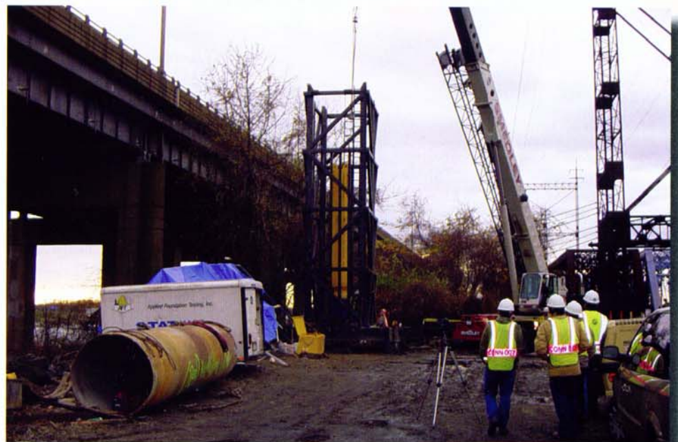
Figure 4: 2000 Ton Statnamic Device with Mechanical Catching System, Stratford, CT
