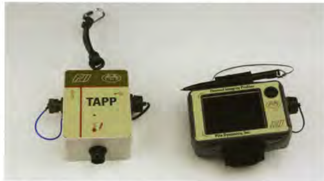
The Thermal Integrity Profiler (TIP).
