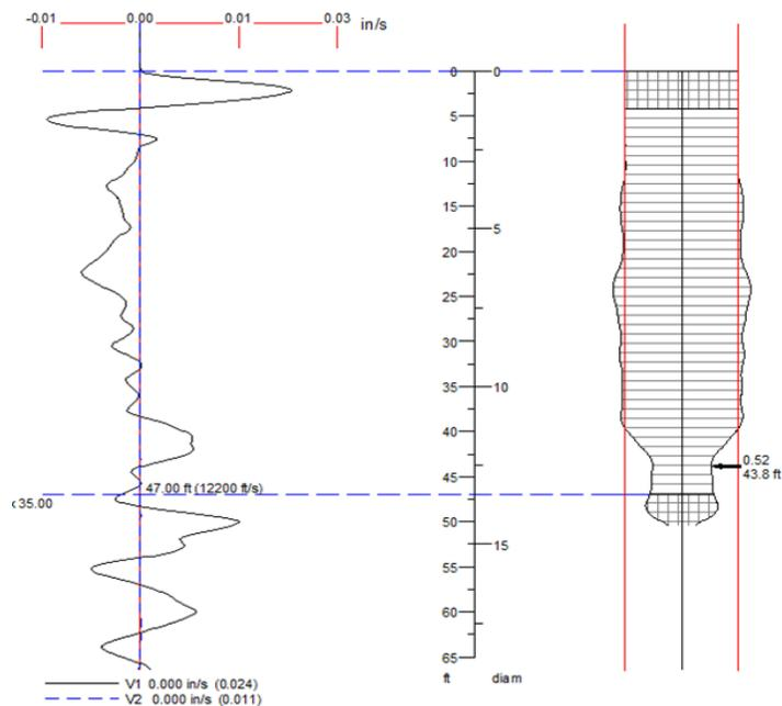
21 **FIGURE 3 Low Strain Test Record and Profile Analysis Result (1 ft = .305 m).**
