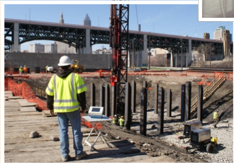
Above: Skylights brighten PDI and GRL lunch room, conserving energy; Left: GRL engineer testing the foundations of the new Innerbelt Bridge, 2011.
