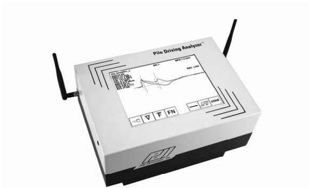
Figure 2: PDA with Antenna
