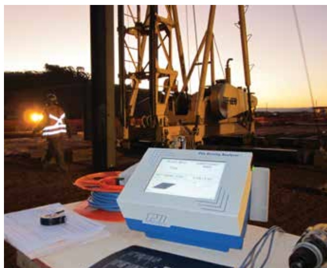
Pile Driving Analyzer
