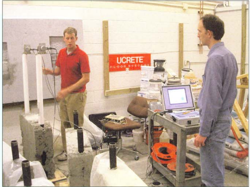
Eric Mack (l), Cleveland State University and Brent Robinson, formerly a GRL engineer who is currently at North Carolina State University, conducting CHA testing on a specimen of conventional concrete.
