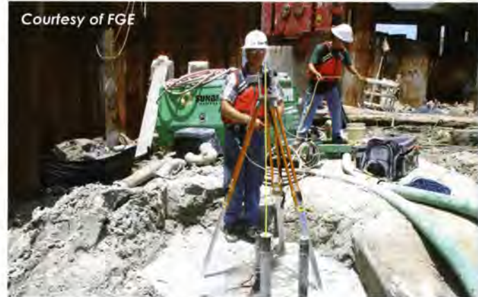
Courtesy of FGE Thermal testing by probe method
