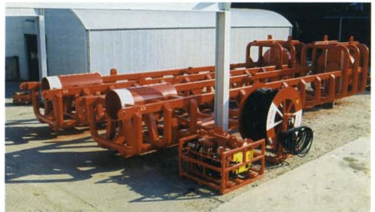
Photo: DELMAG rope suspended leads, power pack and hose drum
