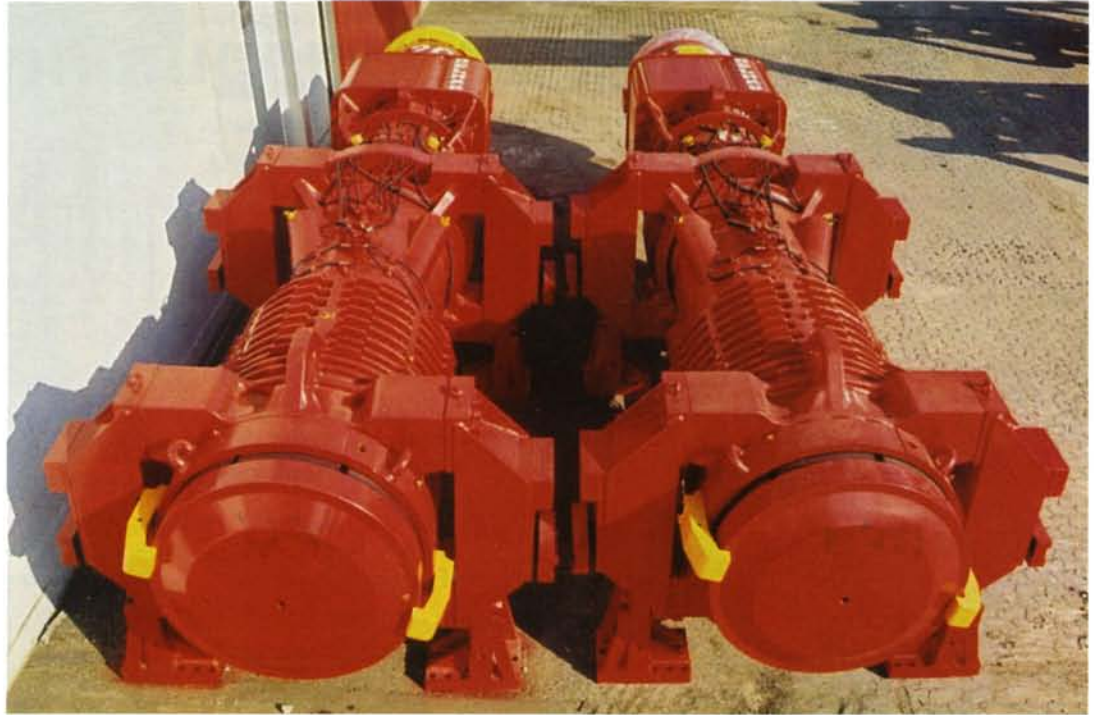
Photo: DELMAG diesel pile hammers D200 bevor delivery
