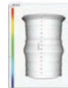
Figure 4 (above): Data from a 22m-long, 45cm-diameter CFA pile
