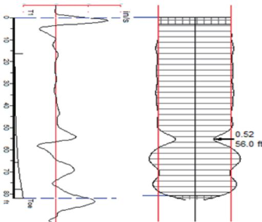
Figure 4. Profile of the defective pile.
