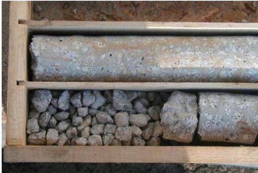
Figure 8. Core of defective shaft showing defect.
