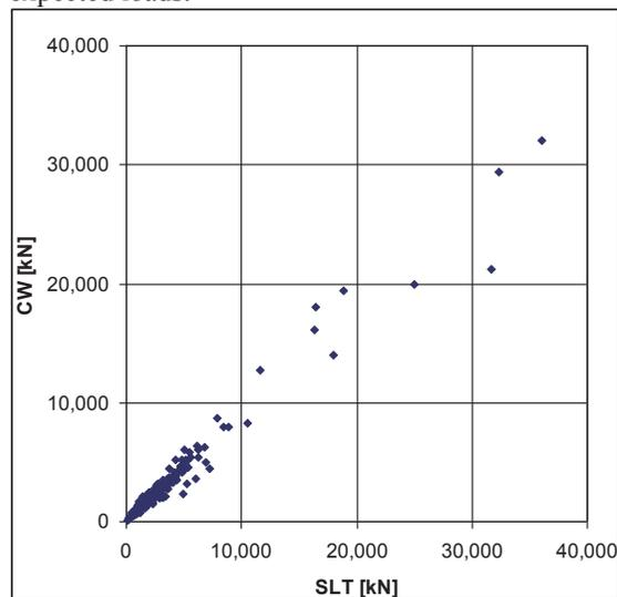
Figure 1. CAPWAP (CW) correlation with Static Load Test (SLT) after Likins and Rausche (2004).
