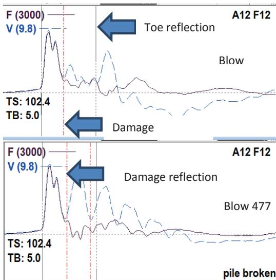
Figure 2. Dynamic testing reveals a pile that is damaged and then breaks completely.
