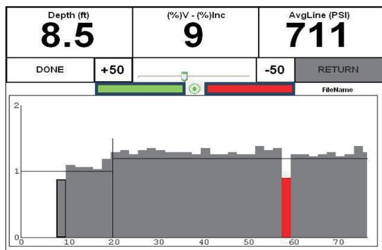
Figure 6. AME screen showing void at 60 feet.
