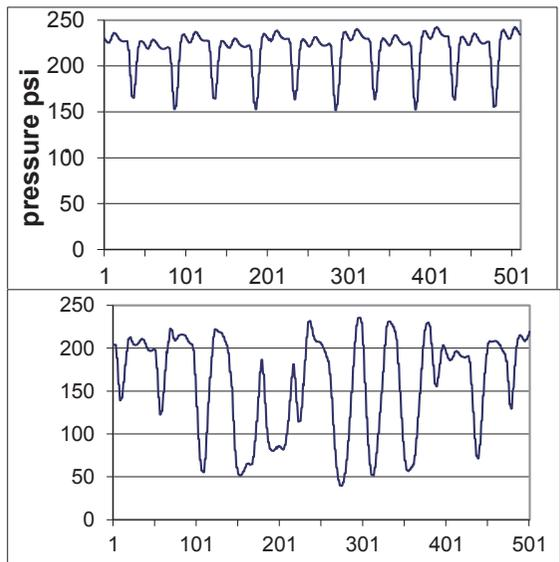
Figure 5. Pressure measurements versus time: top shows normal operation, bottom is faulty pump.
