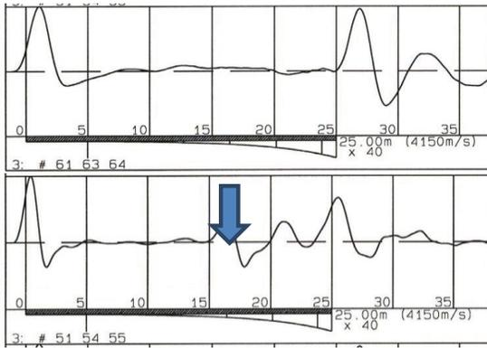
Figure 3. Low strain records of two piles. Top pile is acceptable. Bottom pile has major defect (arrow).
