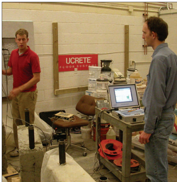
Eric Mack (left), Cleveland State University and Brent Robinson, formerly a GRL engineer who is currently at North Carolina State University, conducting CHA testing on a specimen of conventional concrete.
